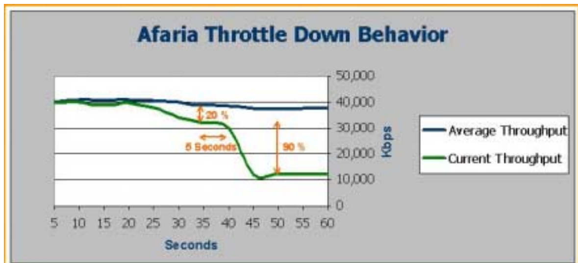
Figure 1.2 – Dynamic Bandwidth Throttling: Sensing and Throttle-down Behavior
